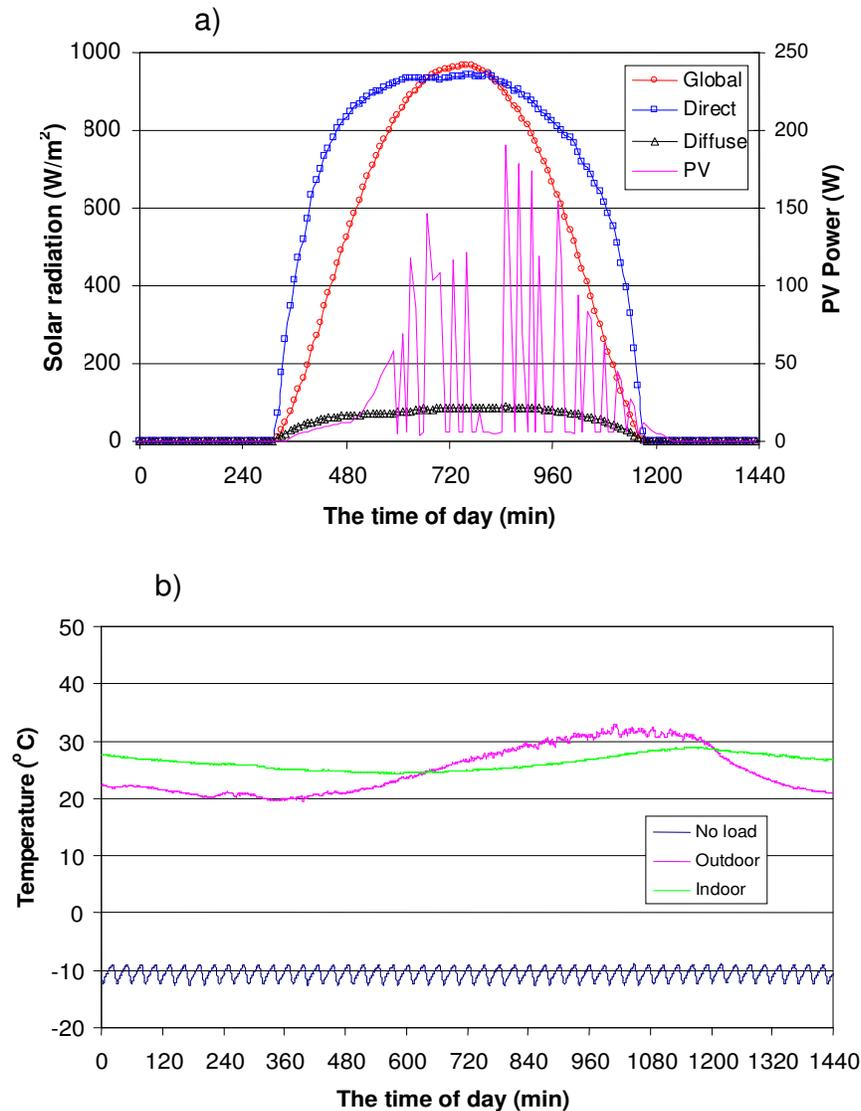
**Figure 3.** Instantaneous values of the some operating parameters for a typical hot day in May 2009, where  $t = 0$  corresponds to local time of 8:00 AM; (a) solar radiation components of global, diffuse and direct, and PV-power, b) temperatures of refrigerator-cabin, room-interior and the ambient.
